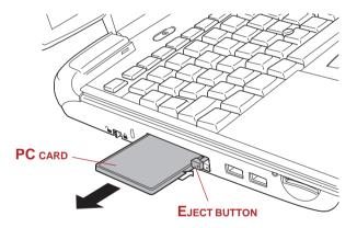
Figure 8-2 Removing the PC card
